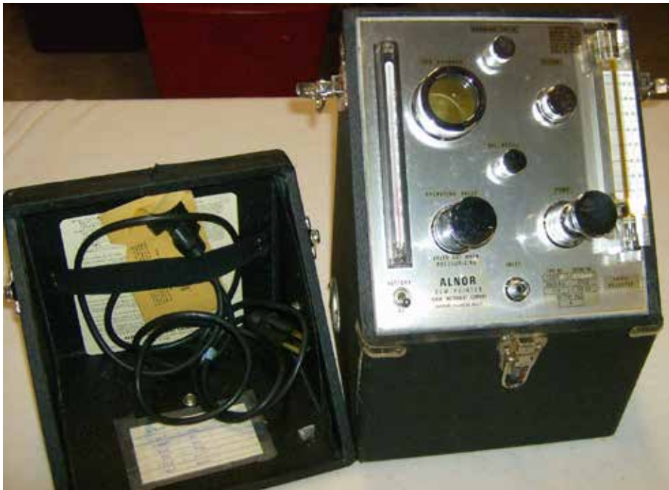
Figure 5: Classic ALNOR Dewpointer used to control carbon potential by the use of water vapor.
