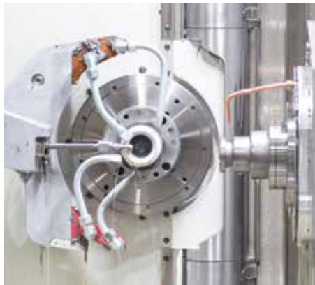
The 280G eliminates pipes, wiring, and clutter from the work area so that swarf containment and evacuation is extremely efficient. Quick-change coolant headers speed setup and ensure optimum coolant delivery.
