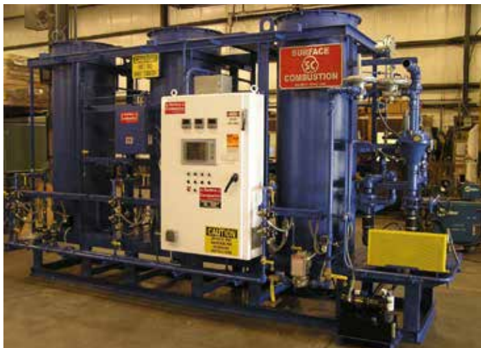
Figure 2: Three retort endothermic generator used to produce endothermic atmospheres. (Courtesy: Surface Combustion, Inc., Maumee, Ohio.)
