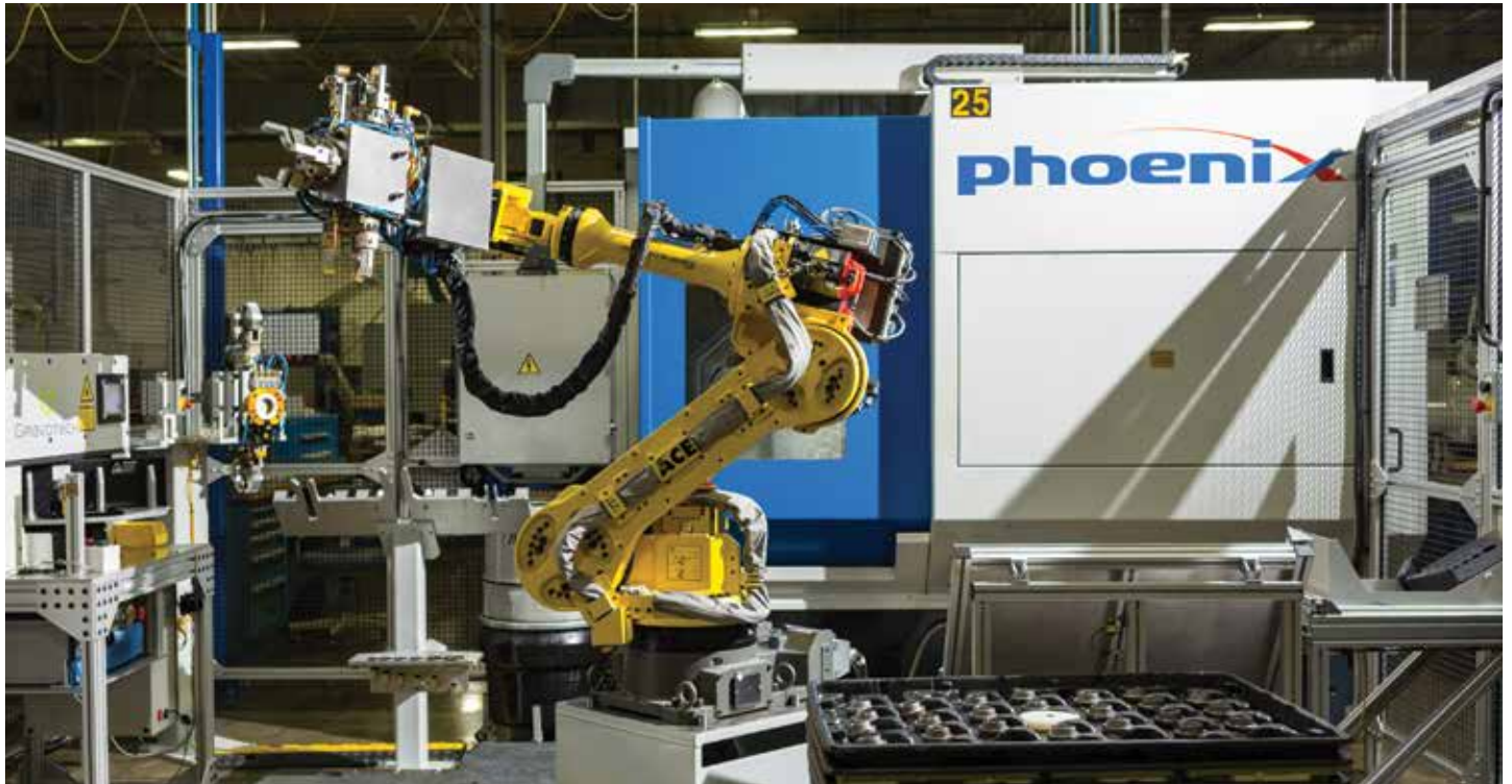
Ten Gleason Phoenix bevel gear cutting machines, including four of Gleason's latest generation of 280CX machines, produce all of the spiral bevel gear sets used in SEW Eurodrive's popular K Series of right-angle gear units.
