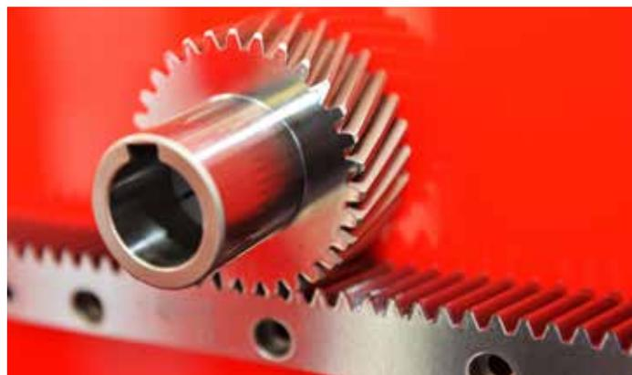
A secondary issue with circular pitch gearing is its relatively infrequent use and the ease at which it is confused with other pitch sizes. The most common accidental interchange is that of CP5 mm and 16DP. These pitch profiles are so similar that many users chose a CP5 pinion but run it against a 16DP rack. This is never a good choice as the rack and pinion will not properly mesh and premature failure due to wear will occur.
