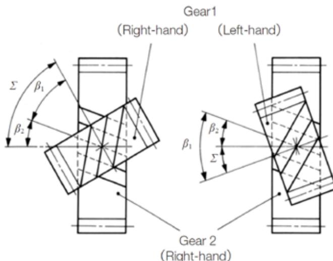
Figure 1: Screw gears of nonparallel and nonintersecting axes.
